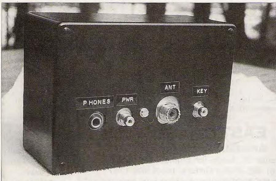
**Photo G.** The rear panel. I should note that the phone jack shown is insulated so that it doesn't provide any connection to the chassis since the receiver 9 VDC power comes through this headphone jack.
